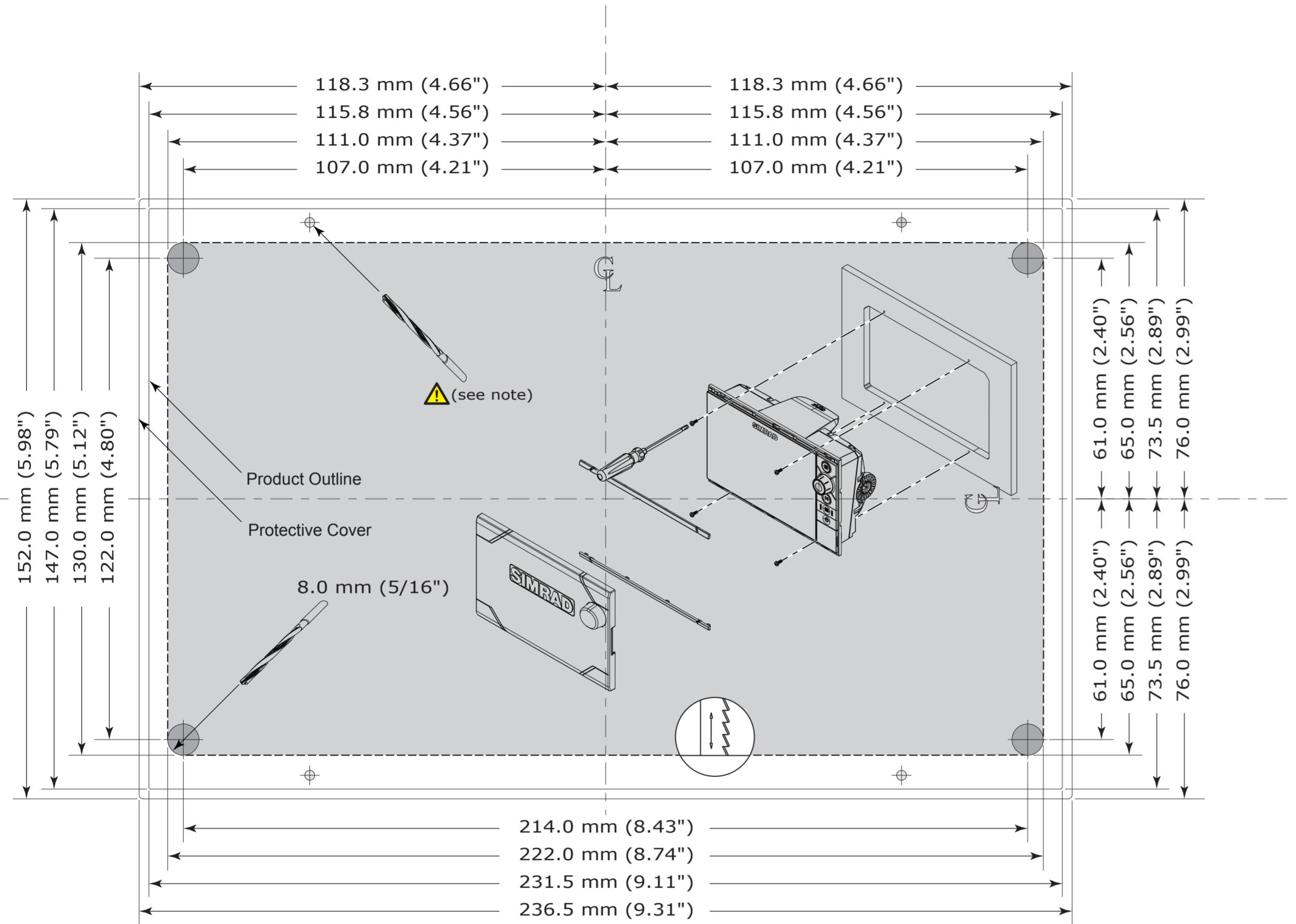
**IMPORTANT.** Do not use this template if it has been rescaled by copying or printing. If this is not the original, or is a print from a file, please check the dimension lines below are to scale before use.
