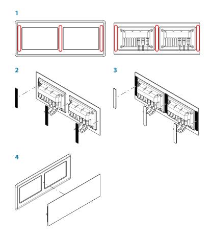
→ Note: The Information Display can be removed from dash by pulling out the glass from the top or bottom side. Support the glass both from the back and the front while removing the glass.
