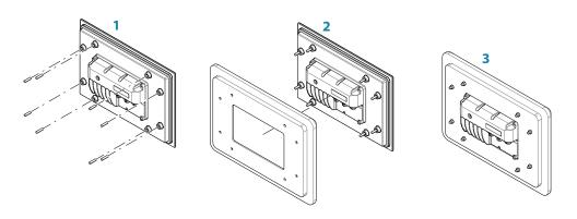
→ Note: If the Information DIsplay(s) has to be removed, make sure to support the glass both from the back and the front while removing the glass.
